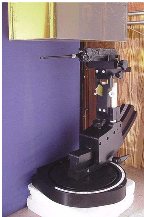
Face-Held SAR Measurement Setup
