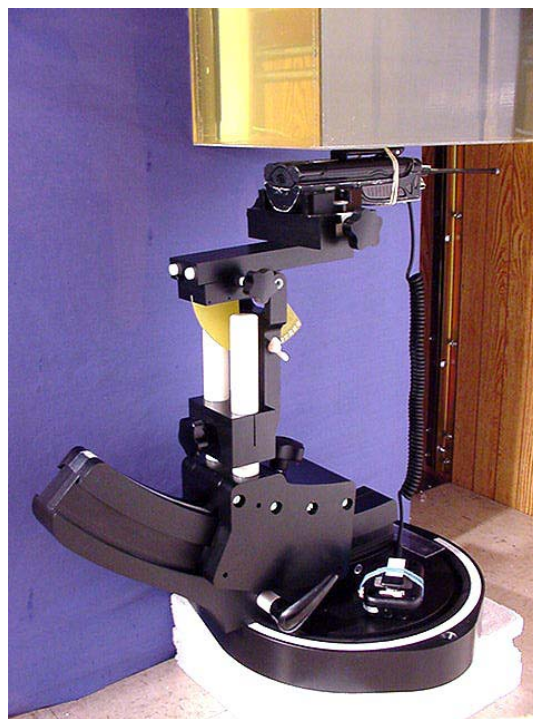
Body-Worn SAR Measurement Setup
