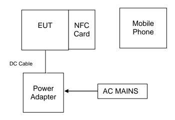
Note: Test was performed with tag and without tag, but only the worst case data (with tag) was recorded in the report.
