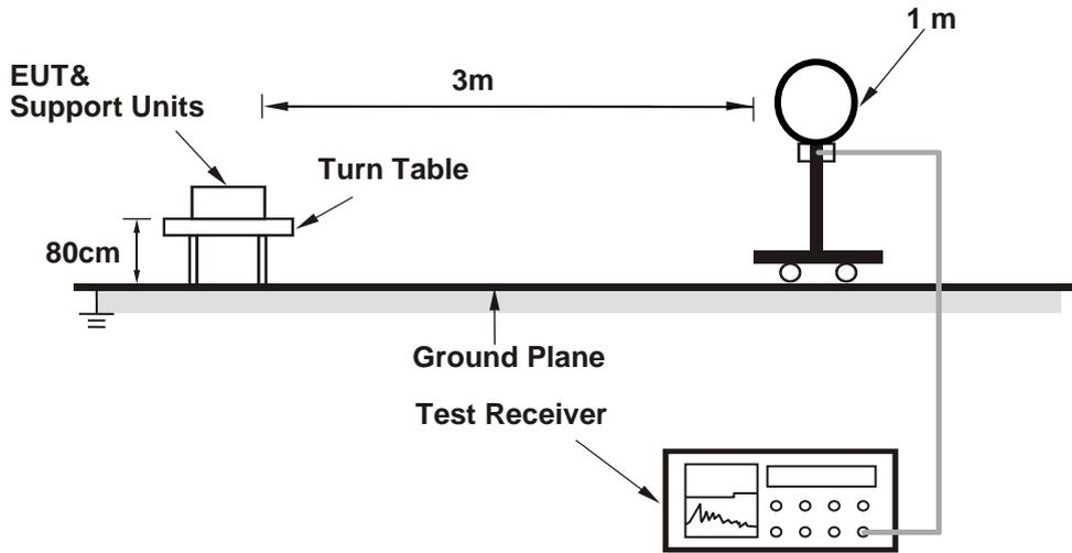
For Radiated emission 30MHz to 1GHz
