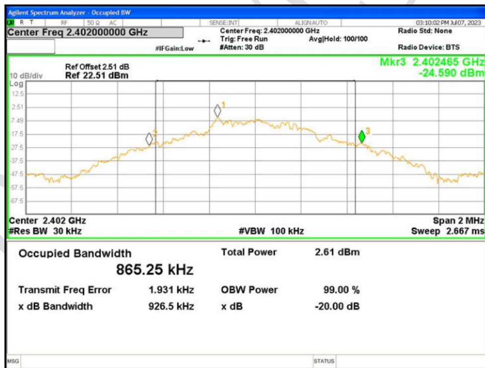
-20dB Bandwidth NVNT 1-DH1 2402MHz Ant1
