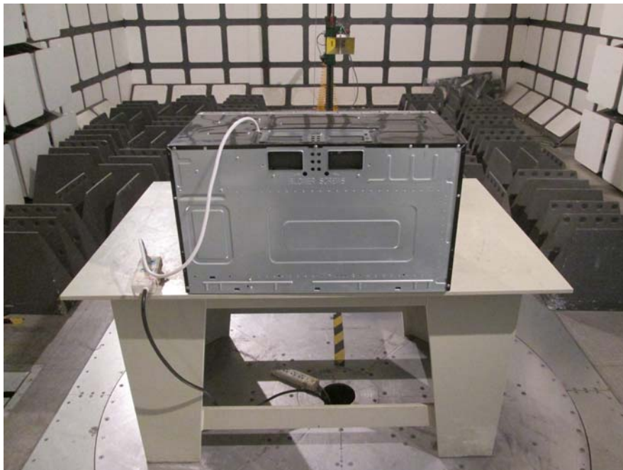
Radiated Emissions - Rear View (Above 1 GHz)
