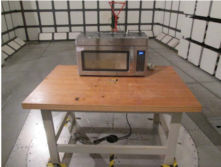
Radiated Emissions - Front View (30 MHz – 1 GHz)
