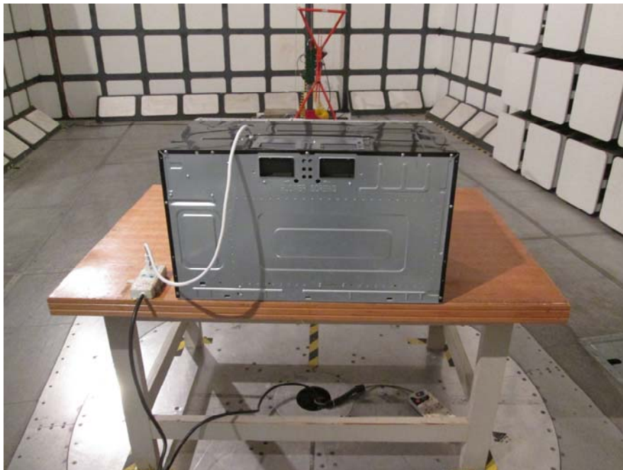
Radiated Emissions - Rear View (30 MHz – 1 GHz)
