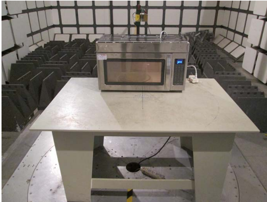
Radiated Emissions - Front View (Above 1 GHz)
