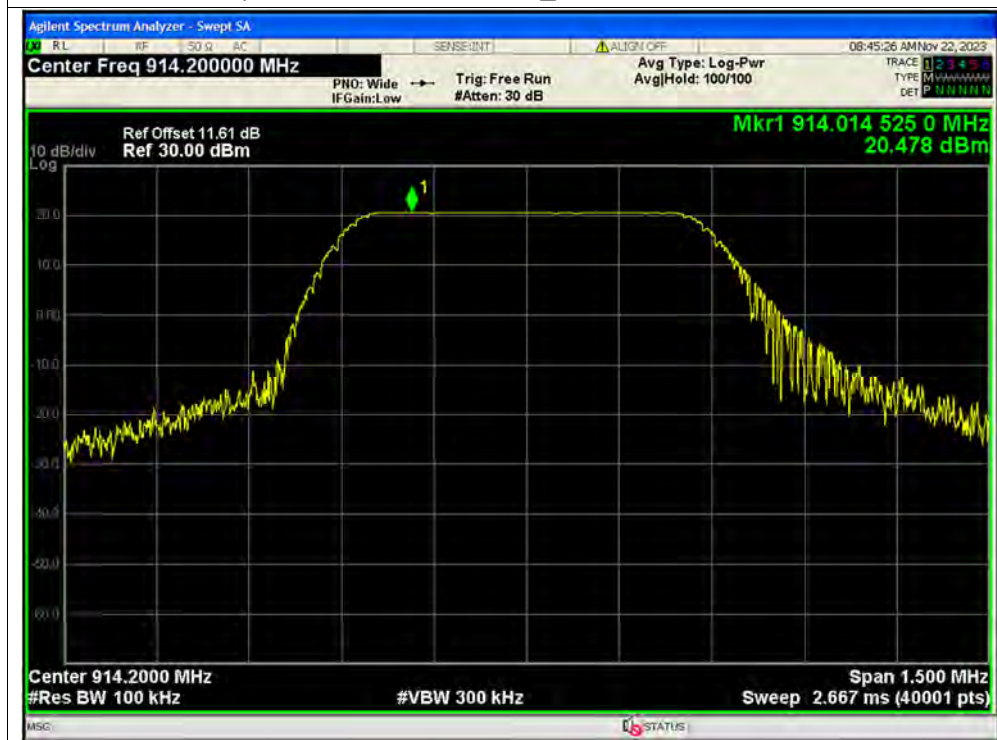
Tx. Spurious NVNT LoRa DTS_SF8 914.2MHz Ant1 Emission
