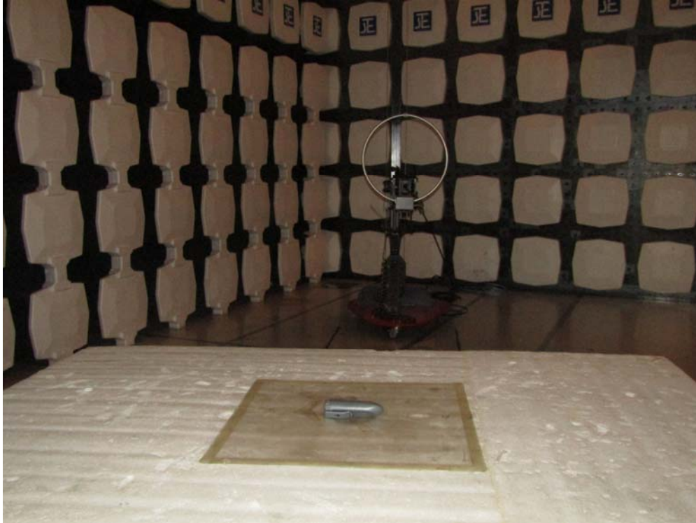
Measurement of Radiated Emission Test Set Up
