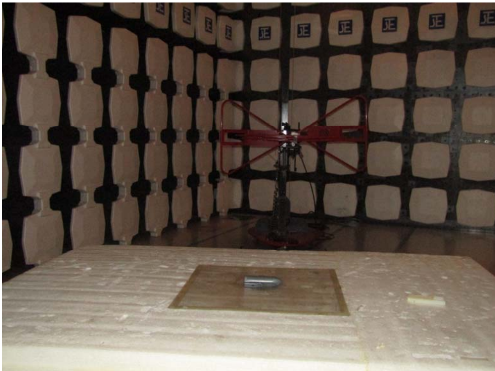
Measurement of Radiated Emission Test Set Up
