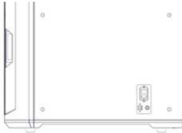
Fig. 5.1 Printer Power Supply Port and Switch
