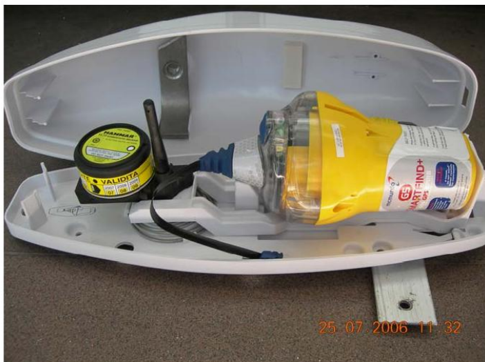
The release mechanism primed ready for the cover to be put on, Hammar H20 release can be seen to the left and when hydrostatically triggered will cut through the black nylon post that holds the cover on. The coiled spring under the hinged release plate will then push up and away the G5 beacon.
