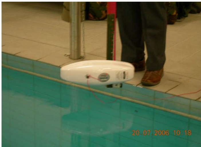
EPIRB mounted on the plunge pole ready test, Rolling 90° attitude.
