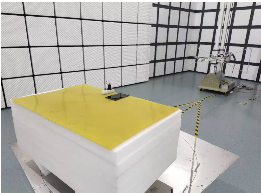
Photo of Radiated Emission Measurement (Above 1G)
