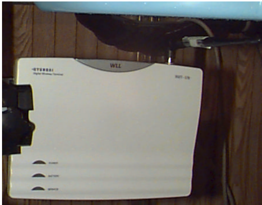
Figure 8. Test setup of EUT in normal operating position with the source of significant emissions (antenna) 2.5 cm below the phantom.
