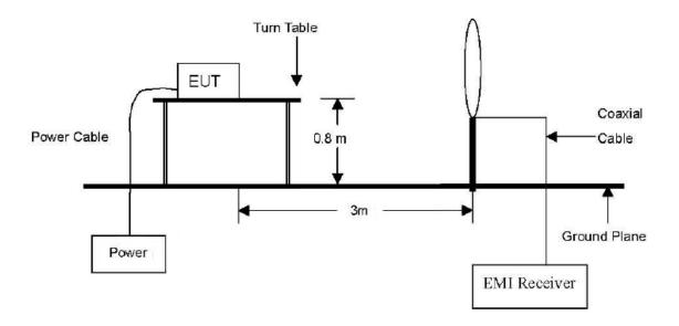
The diagram below shows the test setup that is utilized to make the measurements for emission from 30  $\, \text{Mz} \,$  to 1  $\, \text{GHz} \,$  emissions.
