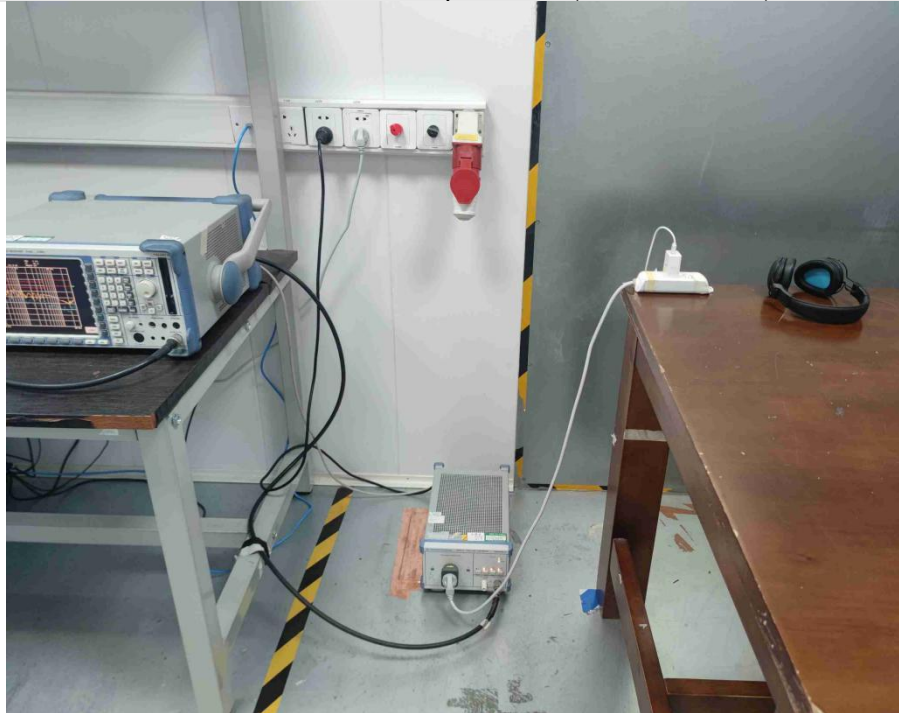
Conducted emissions at AC power line (150kHz-30MHz)
