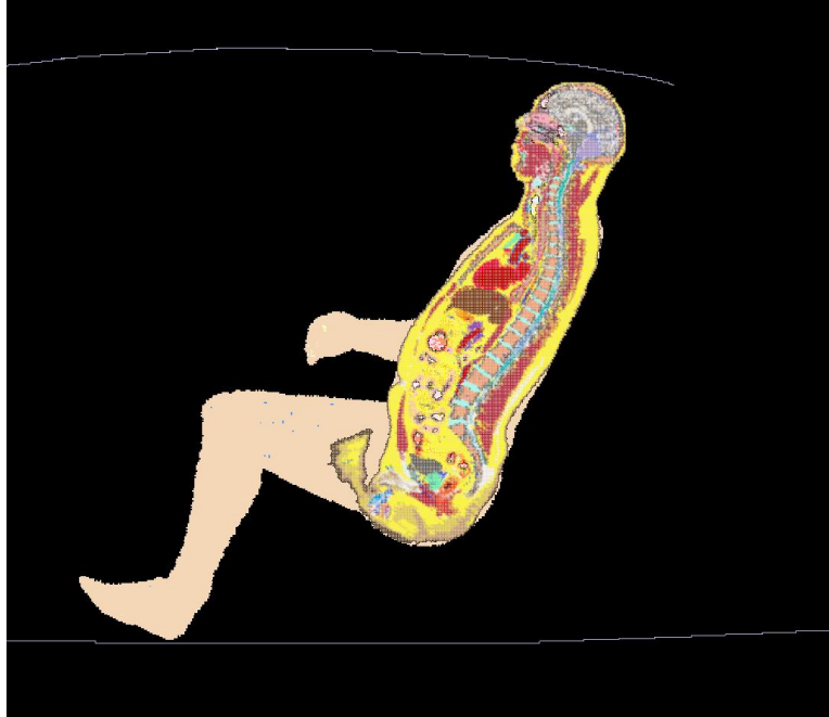
Figure 2: Passenger (back seat) model exposed to a trunk-mount antenna: XFDTD™ geometry. The antenna is installed at 85 cm from the passenger located in the center of the back seat.
