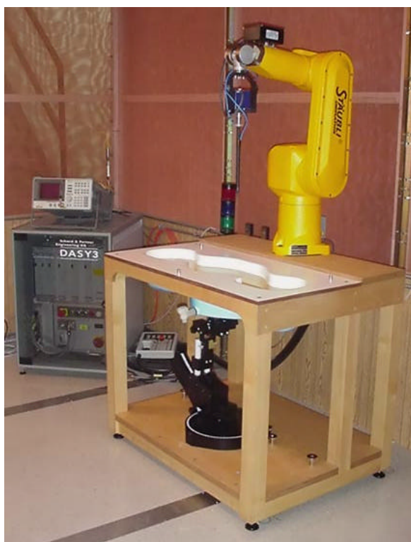
DASY3 SAR Measurement System with Generic Twin Phantom
