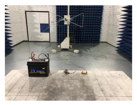
**RADIATED EMISSION TEST SETUP ABOVE 1G**
