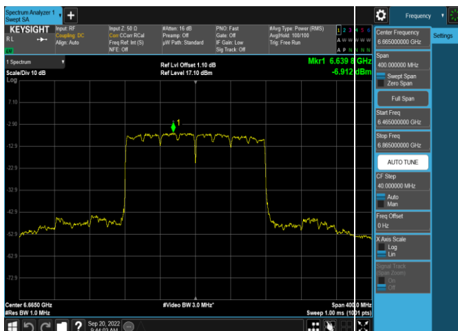
Plot 7-175. Power Spectral Density Plot Antenna 5b (160MHz 802.11ax (UNII Band 7) – Ch. 143, MCS11)
