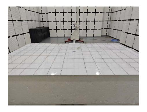
Set-up for Radiated Spurious Emission, Above 1GHz
