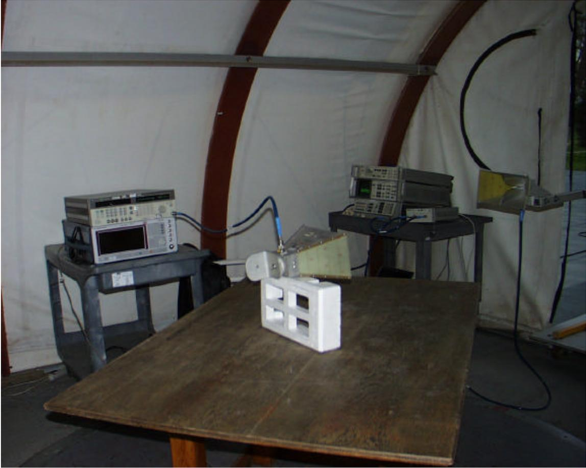
**SUBSTITUTION MEASUREMENT, HORIZONTAL POLARIZATION**
