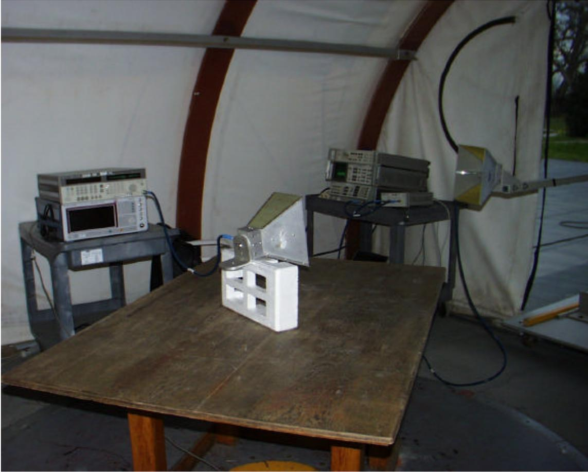
**RADIATED EMISSIONS, LOW FREQUENCY (30-1000) MHz, Front View**
