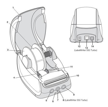
1 Cover USB status light 11 Label guide Label roll Power (On/Off) 12 Power port Printer status light 8 LAN status light 13 LAN port Label spool (LabelWriter 550 Turbo) (LabelWriter 550 Turbo) Label release lever Label forward feed 14 USB port Label reverse feed 10 Label exit slot and tear bar
