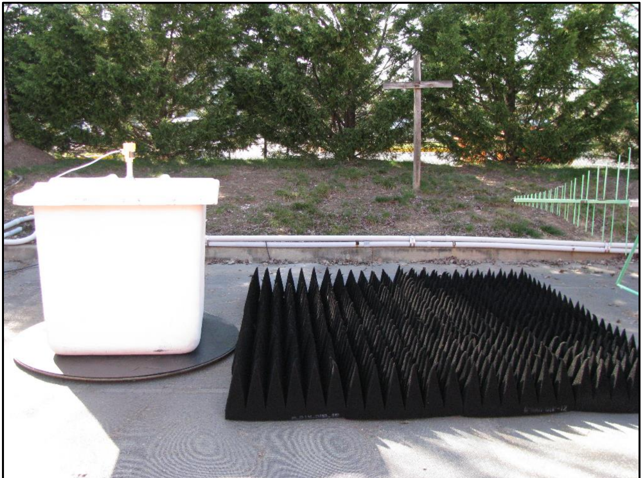
Photograph 62: Radiated Emissions – TC #7; Fiberglass Container, Rear View
