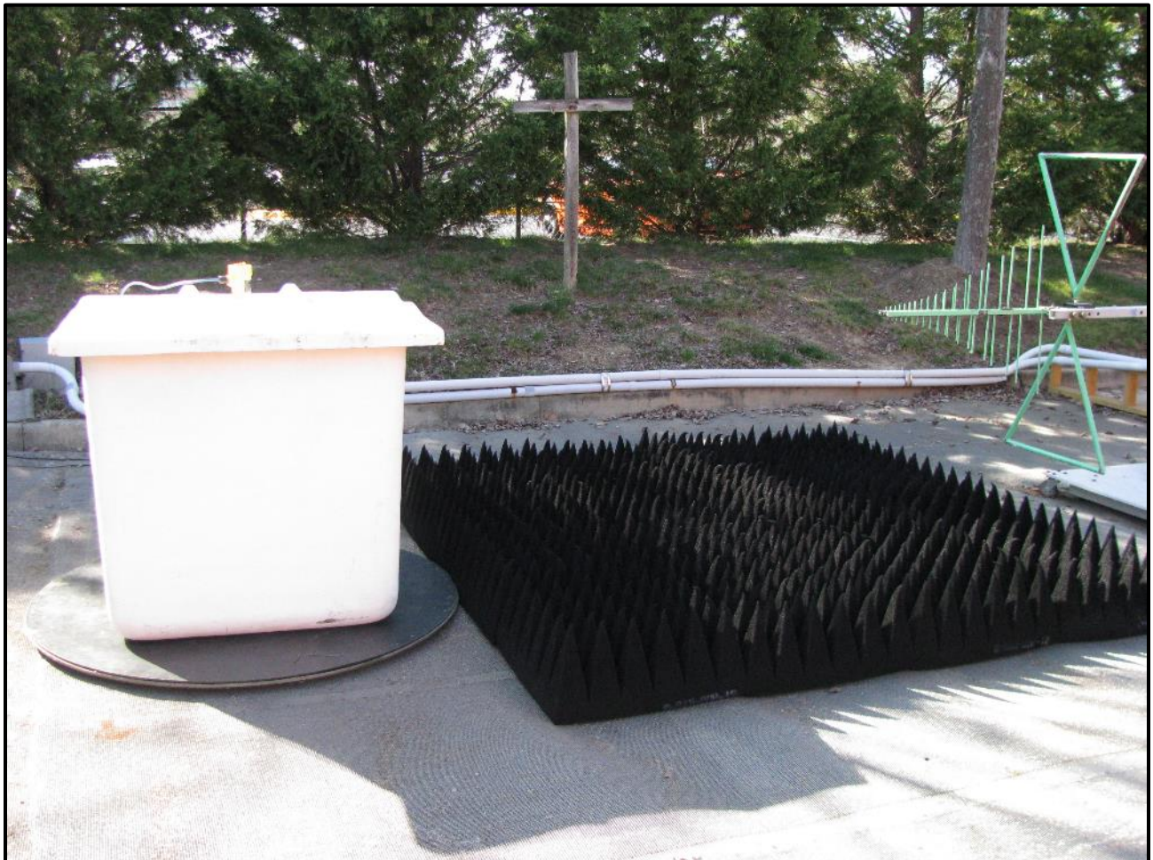
Photograph 56: Radiated Emissions – TC #4; Fiberglass Container, Rear View
