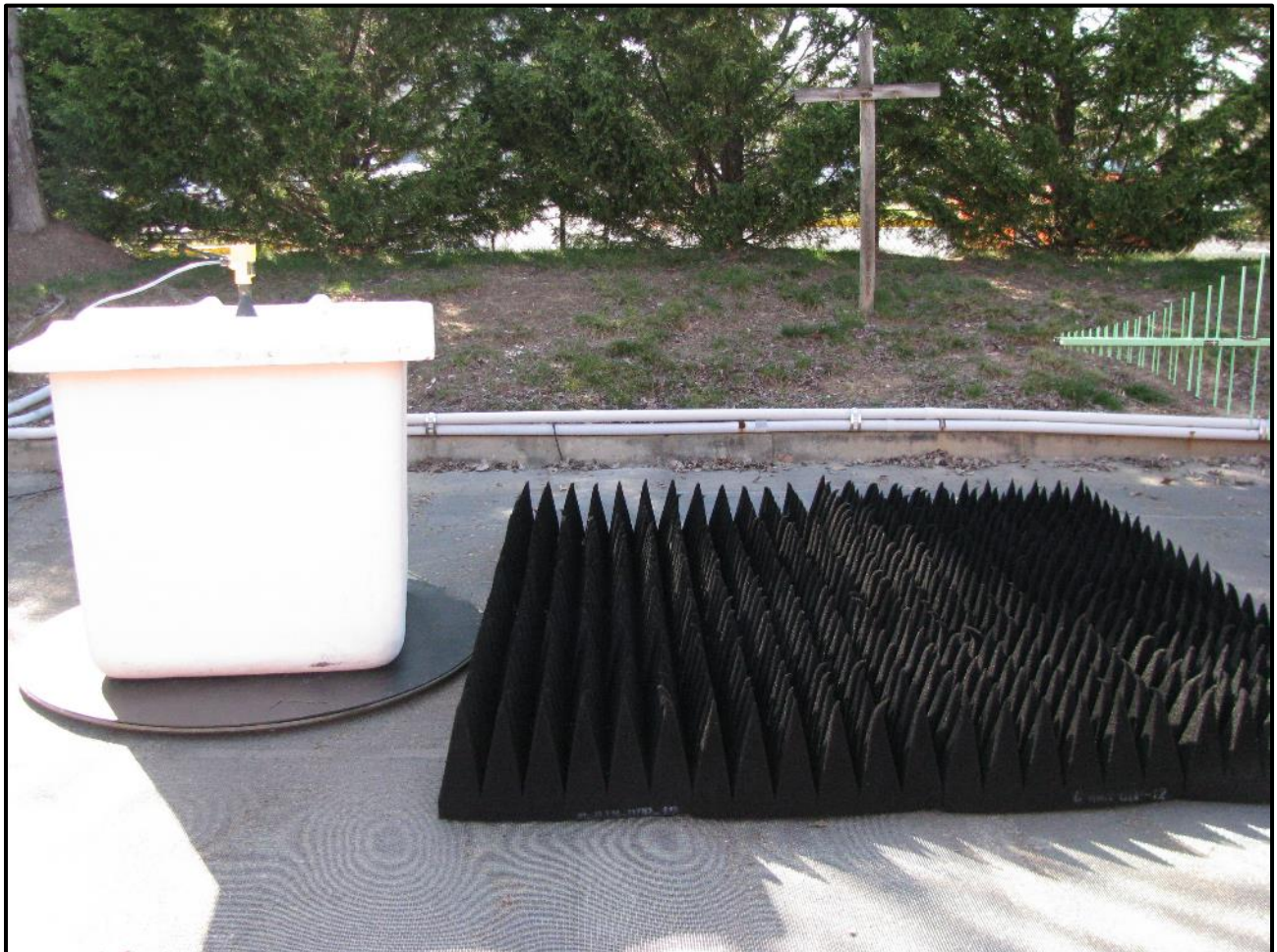
Photograph 50: Radiated Emissions – TC #1; Fiberglass Container, Rear View
