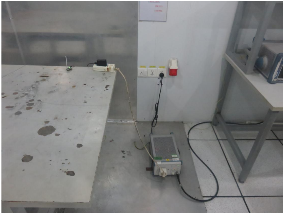
Photo of Conducted Emission Measurement
