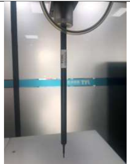
Fig.8.2 Photo of E-Field Probe
