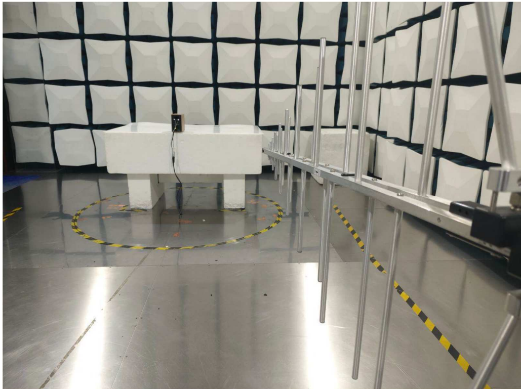
Photograph 2: Set-up for Radiated Spurious Emission, below 1GHz
