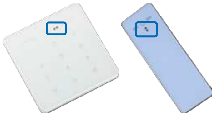
Fig. 6 - proximity and ambient light sensors (blue frames) Secustos SQ80 (left) and MU20 (right) reader models
