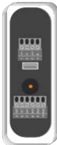
Fig. 9 - connectors on Secustos MU20 reader models
