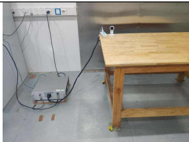
Conducted Emissions Test Setup Front View
