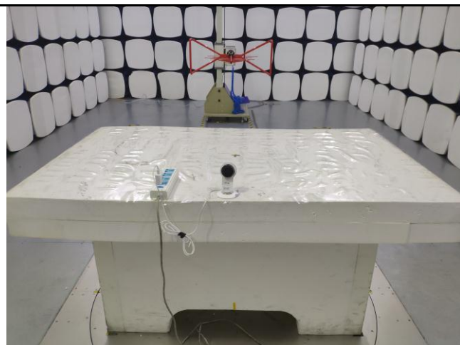
Radiated Spurious Emissions Test Setup Below 1GHz
