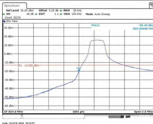
Band26 3MHz 16QAM 26805 15RB#0
