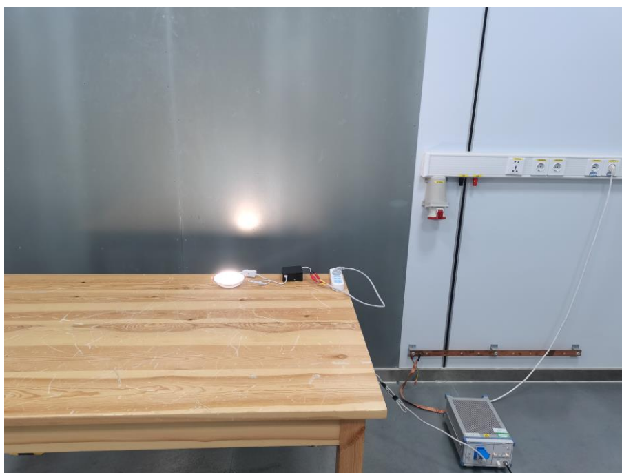
Fig. 4 Power line conducted emission setup photo
