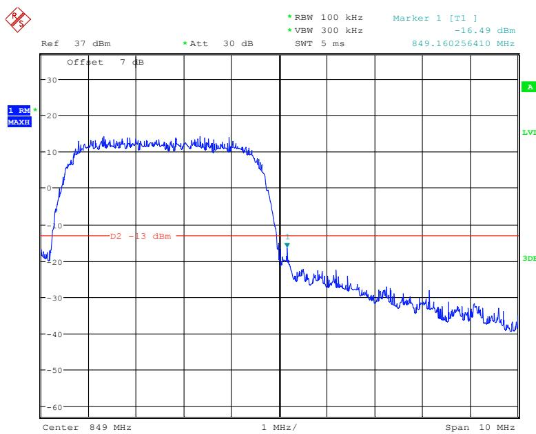
**PCS Band, Left Band Edge for GSM (GMSK) Mode**
