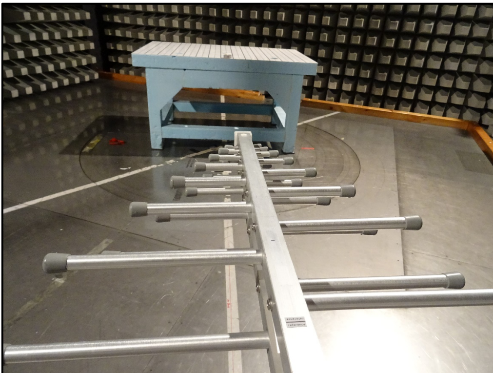
Photo 5: Radiated Test Setup -30 MHz to 1GHz EUT
