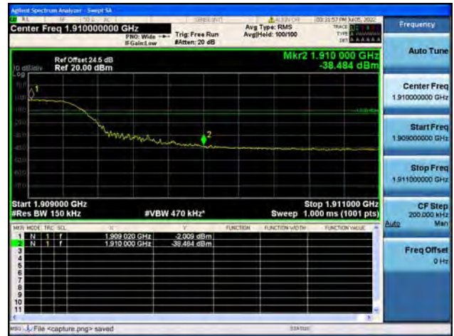
Band2 / 15MHz / High CH / QPSK / FULL RB
