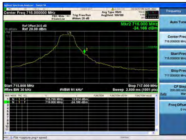
Band12 / 3MHz / High CH / QPSK / 1 RB
