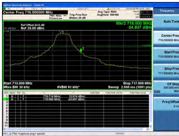
Band12 / 1.4MHz / High CH / QPSK / 1 RB
