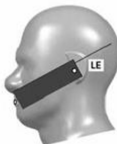
Picture15 Handset vertical and horizontal reference lines—"clam-shell case"
