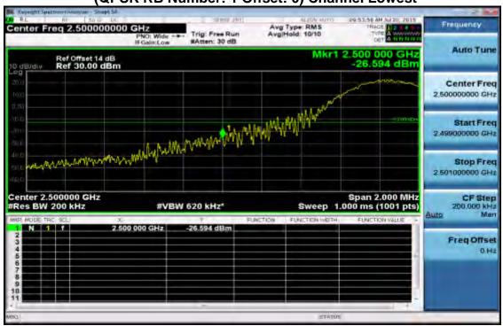
Band edge emission at antenna terminals -15MHz BW LTE-Band 7 (QPSK RB Number: 1 Offset: 74) Channel Highest
