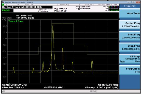
Emission Mask at antenna terminals -10MHz BW LTE-Band 7 (QPSK RB Number: 1 Offset: 49) Channel Lowest
