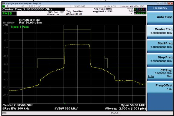
Emission Mask at antenna terminals -10MHz BW LTE-Band 7 (QPSK RB Number: 50 Offset: 0) Channel Mid
