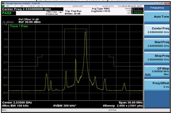
Emission Mask at antenna terminals -5MHz BW LTE-Band 7 (QPSK RB Number: 1 Offset: 24) Channel Highest
