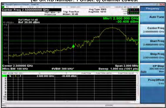
Band edge emission at antenna terminals -10MHz BW LTE-Band 7 (QPSK RB Number: 1 Offset: 49) Channel Highest
