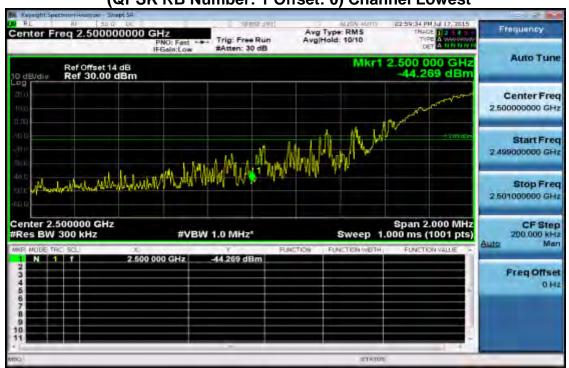
Band edge emission at antenna terminals -20MHz BW LTE-Band 7 (QPSK RB Number: 1 Offset: 99) Channel Highest
