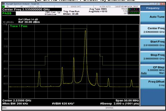
Emission Mask at antenna terminals -10MHz BW LTE-Band 7 (QPSK RB Number: 1 Offset: 49) Channel Highest
