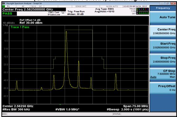
Emission Mask at antenna terminals -15MHz BW LTE-Band 7 (QPSK RB Number: 1 Offset: 74) Channel Lowest
