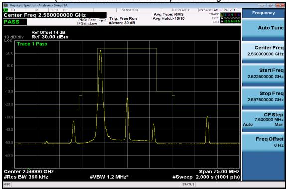
Emission Mask at antenna terminals -20MHz BW LTE-Band 7 (QPSK RB Number: 1 Offset: 99) Channel Lowest
