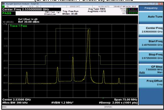
Emission Mask at antenna terminals -20MHz BW LTE-Band 7 (QPSK RB Number: 1 Offset: 99) Channel Highest
