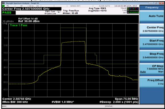
Emission Mask at antenna terminals -15MHz BW LTE-Band 7 (QPSK RB Number: 75 Offset: 0) Channel Mid
