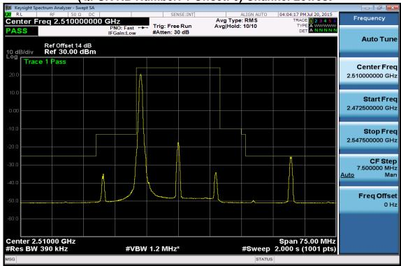
Emission Mask at antenna terminals -20MHz BW LTE-Band 7 (QPSK RB Number: 1 Offset: 0) Channel Mid
