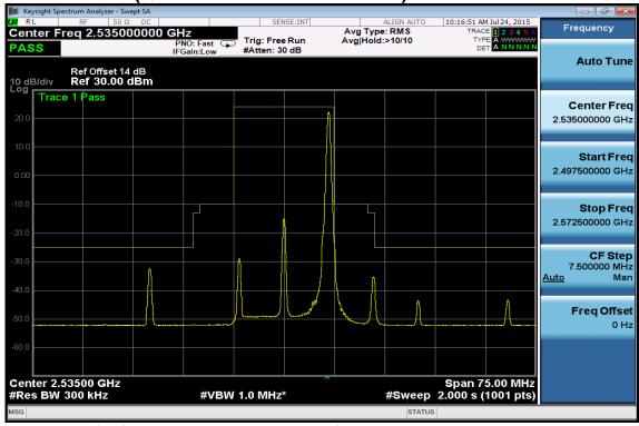
Emission Mask at antenna terminals -15MHz BW LTE-Band 7 (QPSK RB Number: 1 Offset: 74) Channel Highest
