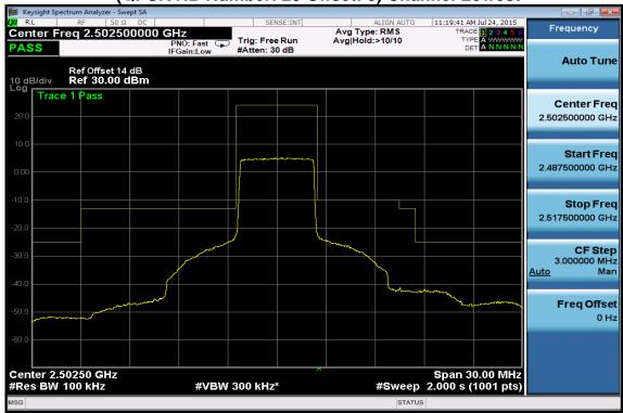
Emission Mask at antenna terminals -5MHz BW LTE-Band 7 (QPSK RB Number: 25 Offset: 0) Channel Mid
