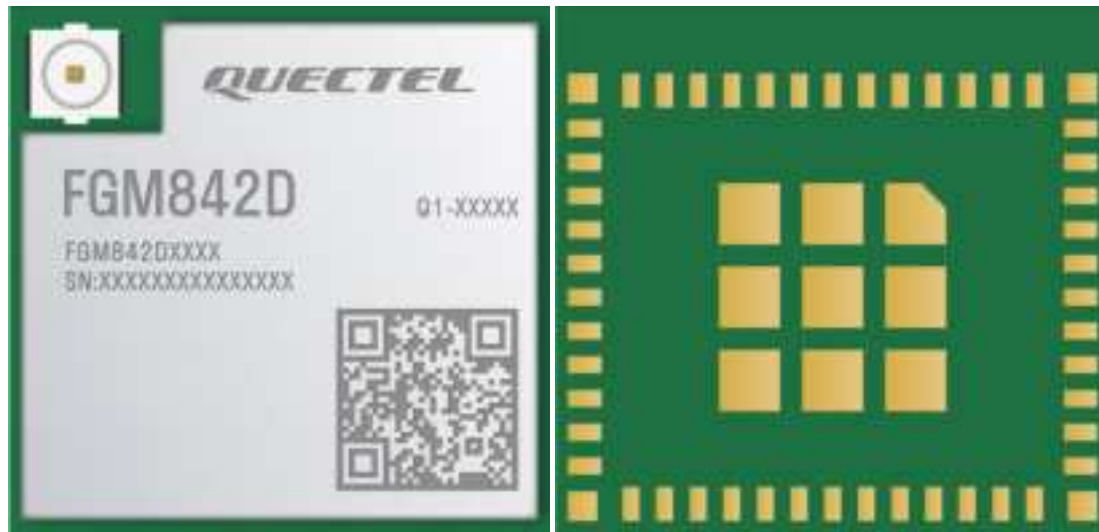
Figure 18: FGM842D Top and Bottom Views
