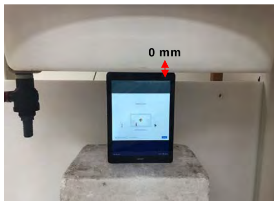
Fig.4 EUT Top side to flat phantom
