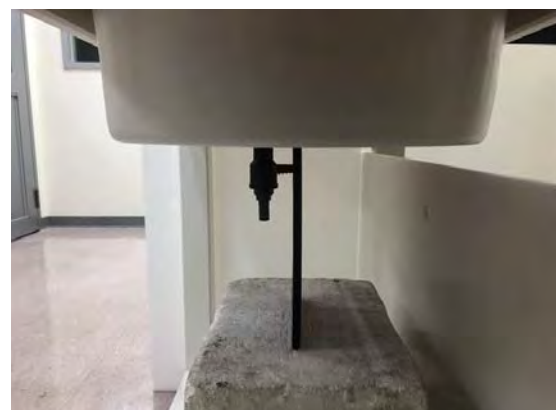
Fig.4 EUT Top side to flat phantom
