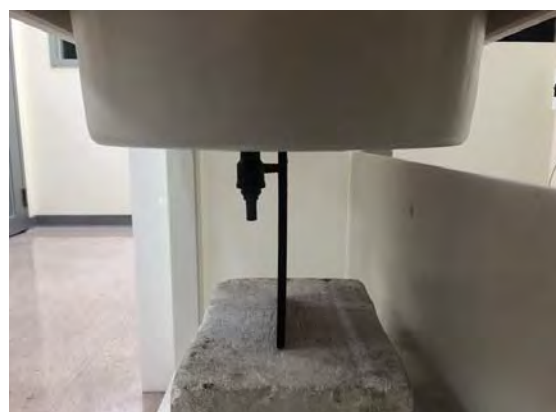
Fig.7 EUT Bottom side to flat phantom
