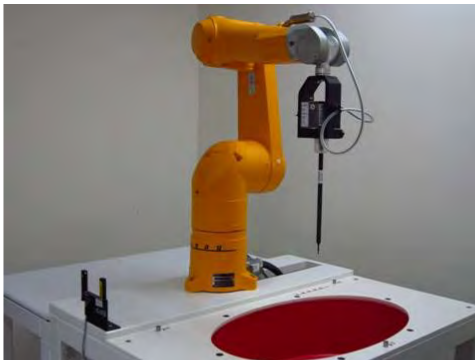
Fig.1 Photograph of the SAR measurement system
