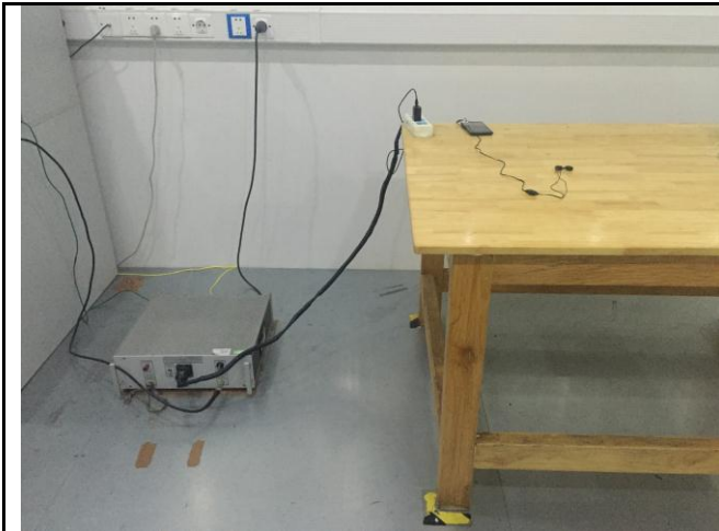
Conducted Emissions Test Setup Front View
