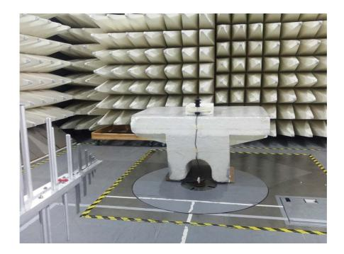
Photograph No.4 Setup for spurious emission measurements in the anechoic chamber below 1000 MHz, EUT close view
