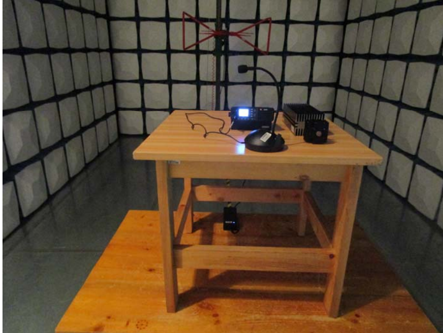
Radiated Emission View (Above 1 GHz) Desk Mounted
