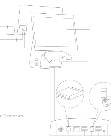
Pull the printer handle out, and the paper roller cover pops out automatically.
