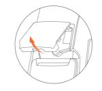
Firstly, open outward the cover of the printer cutter
