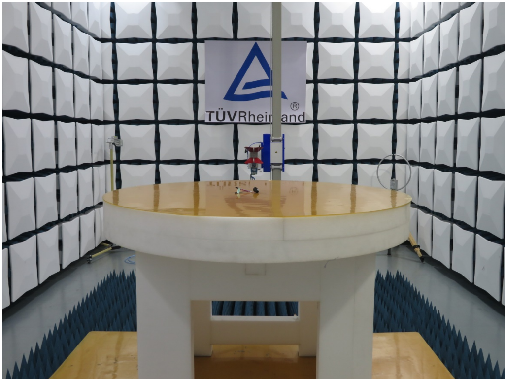
Photograph 2: Set-up for Radiated Spurious Emission, Above 1GHz
