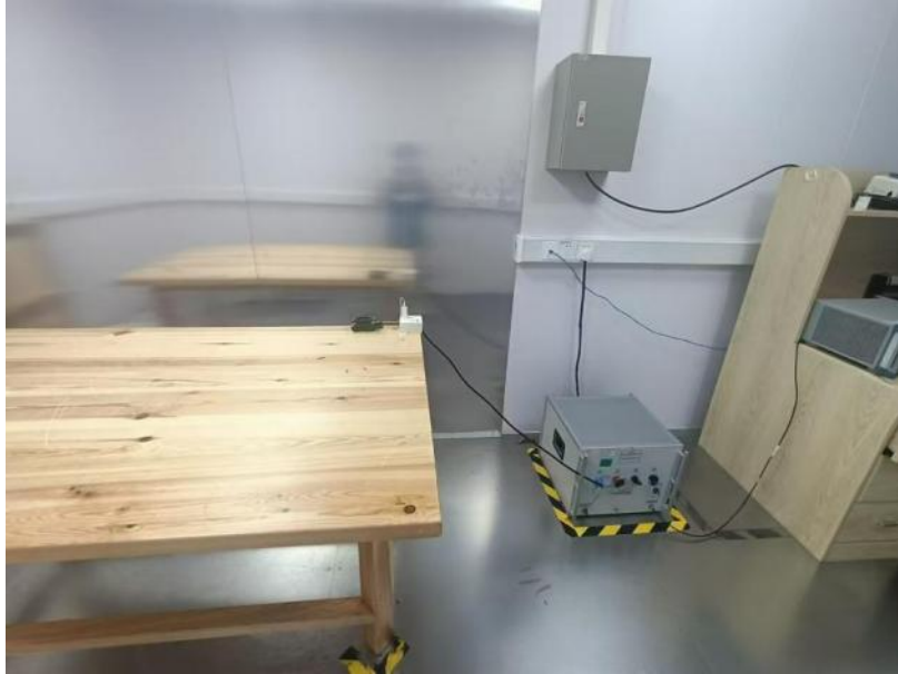
Radiated Emissions From 30M-1GHz
