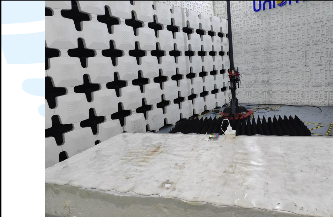
Radiated emission Test Setup-2 (Above 1 GHz)
