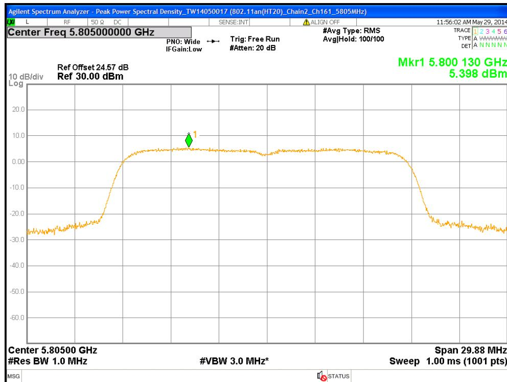
**Chain0 : Peak Power Spectral Density @ 802.11an(HT40) Mode Ch38**
