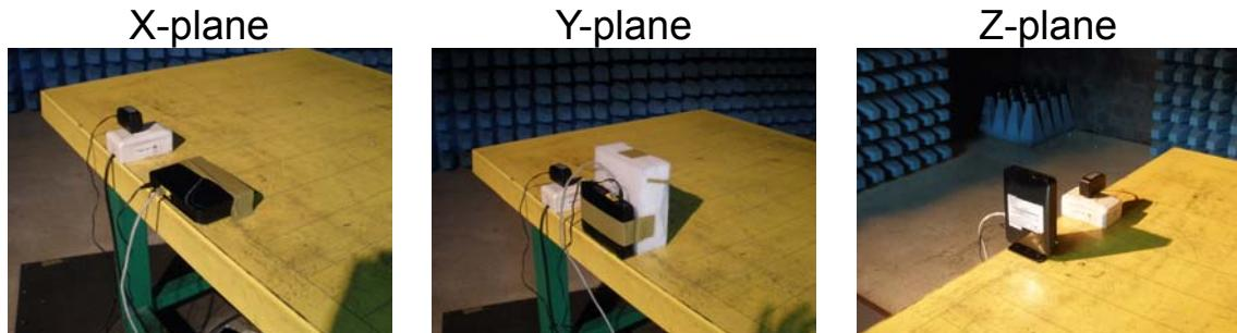
After verifying three axes, we found the maximum electromagnetic field was occurred at Y-plane configuration. The final test data was executed under this configuration.
