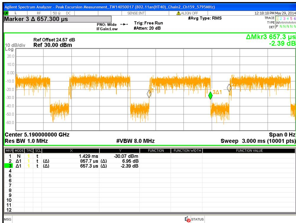
**Chain 0: Duty cycle @ 802.11n(HT40) Mode Channel 151**
