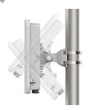
Align Radio to required angle by tilting up and down. The maximum radio tilting angle is ± 40°, with an incremental of 10°.
