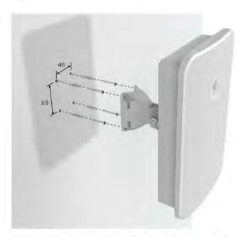
Drill 4 holes of Ø6mm (Ø0.25"Inch) on wall. Press fit plastic anchor and assembly fastener. Leave 5mm to 6mm gap between wall and fastener head. Use the four mounting slots given on the back of the radio to mount to the wall.
