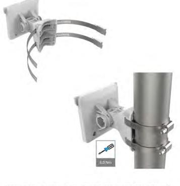
Insert hose clamps through pole mounting bracket and clamp to pole by applying 3.0 Nm torque.
