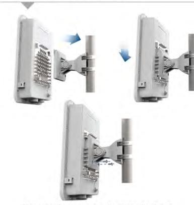
Align the radio chassis with the guide rails of radio holder and slide it downwards until it clicks into place.
