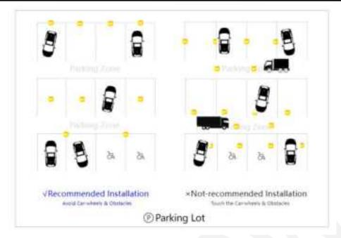
\*The MBM03 beacon is a Bluetooth ® beacon rather than a real road stud. In order to ensure the device performance, please deploy it in the recommended way above as much as possible to prevent the equipment from being repeatedly rolled by vehicles often. Also, considering different users has different scenarios, please contact our sales team if you have any questions about deployment.
