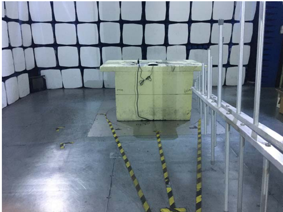
Radiation Emission Test Setup (30MHz to 1GHz)
