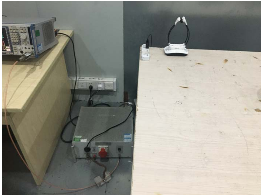
Conducted Emission Test Setup
