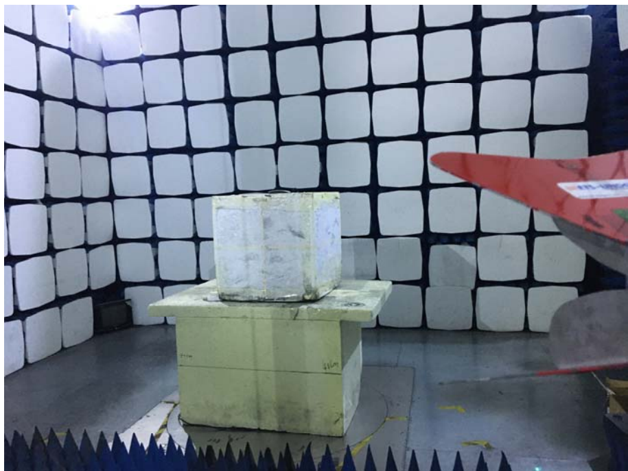
Radiation Emission Test Setup (1GHz to 18GHz)
