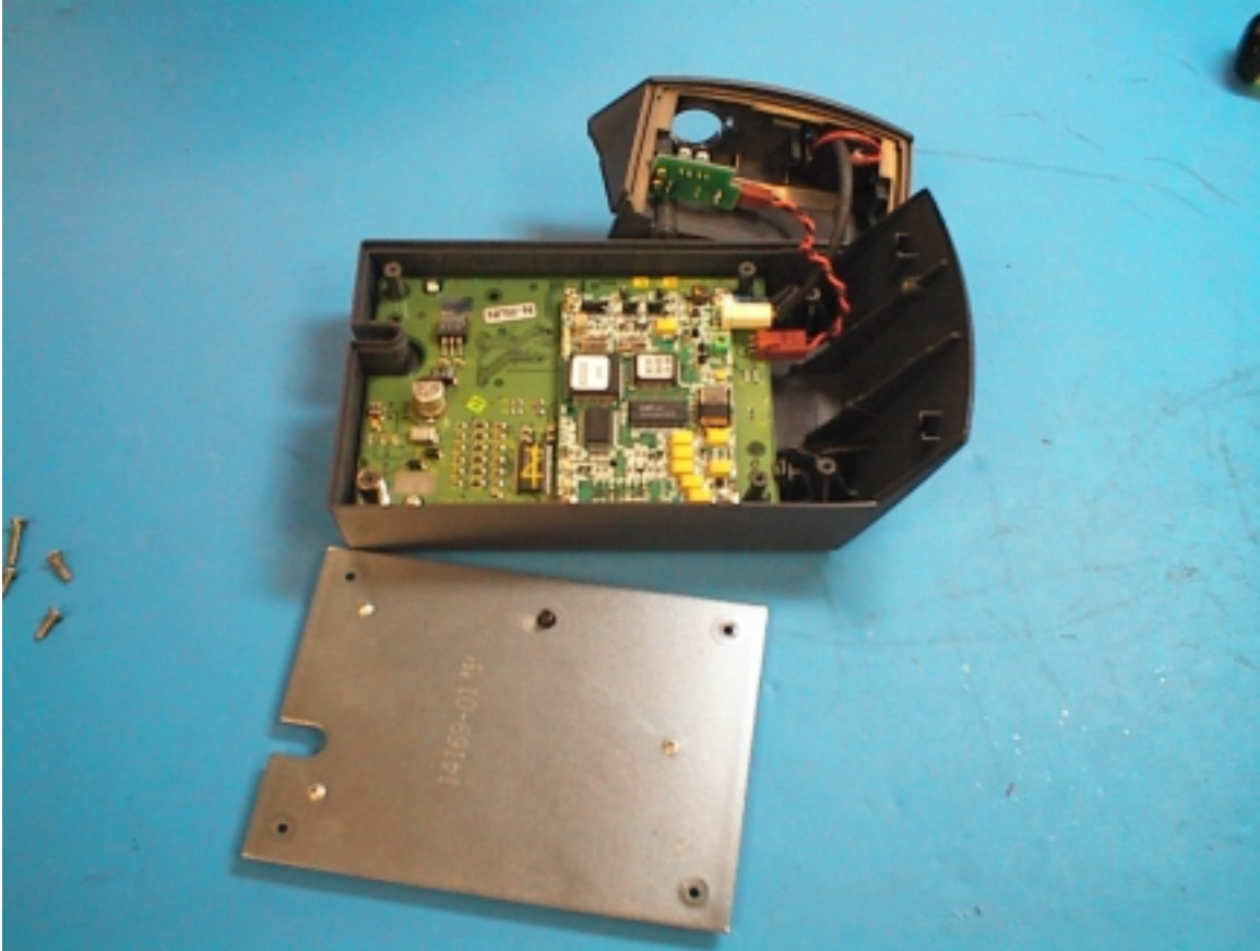
Photo 2 – Disassembled, showing LED PC board and antenna mounting
