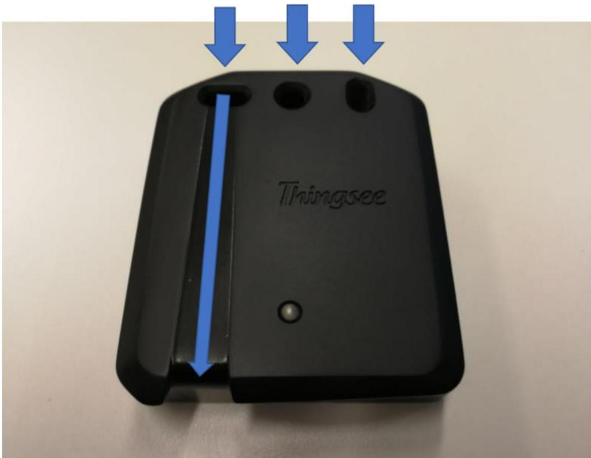
Connect the power source to the gateway and plug it on into the wall socket with 24/7 power.
