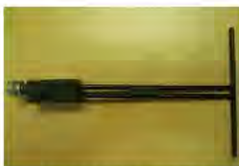
Figure 1 – MVG COMOSAR Validation Dipole
