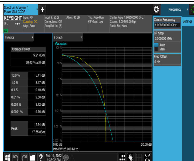
Band2-3MHz-16QAM-19185-6-0-Low-9.19-<=13-PASS
