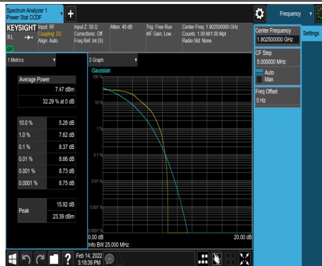
Band2-15MHz-QPSK-19125-6-0-Low-8.37-<=13-PASS
